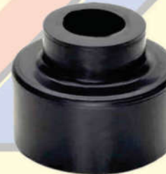
6222 012 - MB271 Bucha do tensor susp. dianteira F-4000 75...98/F-2000 80...85 F-350 72...85/F-400 75...77 Troller T4 99...
