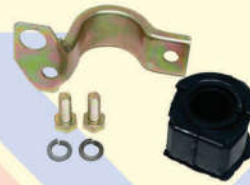
5600 815 1 Rep. barra estab. diant. dir. (furo 23mm) - Strada 97... Palio Weekend 1.0/1.5/1.6 Inclusive 8/16v 97...
