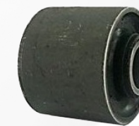
6200 852 Bucha inf. diant.com capa de ferro Nissan Frontier SEL 08...16 amort. Cofap 38mm
